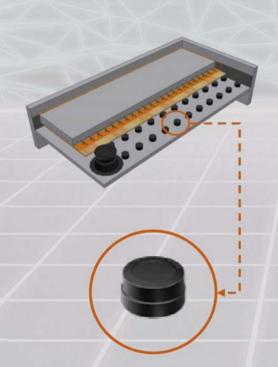
Cylindrical neoprene mountings with a diameter no less than 0.9 of the 2 inch (50mm) height. Isolators are molded to DuPont neoprene AASHO bridge bearing of maximum durometer 60.
